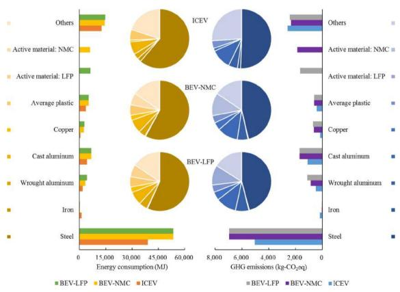
Fig. 4. Energy consumption and GHG emissions of each material.
