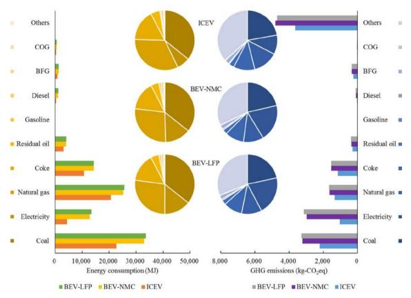
Fig. 5. Energy consumption and GHG emissions of each energy source.
