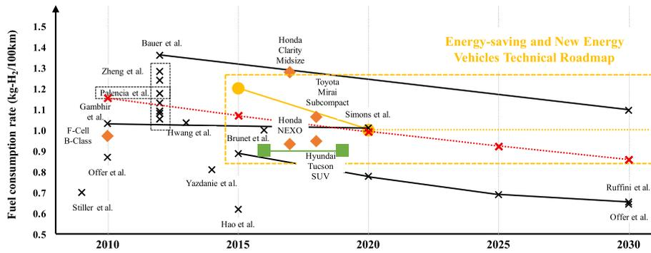
**Fig. 7 – Summary of fuel consumption rates of fuel cell PVs. Supplementary notes: 1 Green marks represent targets set by EU pilot projects. 2 Orange marks represent data from existing fuel cell passenger vehicle models provided by automakers. 3 Yellow marks represent status quo and targets set by the Chinese government. 4 Cross are data from literature review.**
