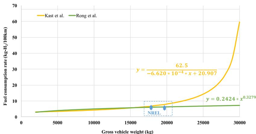
(b) ICE and fuel cell commercial vehicle fuel economy re-fitted curve as a function of gross vehicle weight
